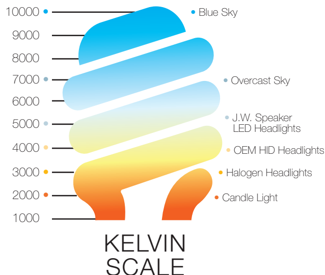
Color temperature does not measure or indicate the physical heat coming from a light source.
